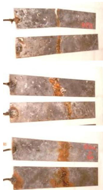
Figure 1.4: Visual observation of the corrosive attack at the crack apex on bare steel plates embedded in natural-aggregate concrete (above), RAC (middle) and HVFA concrete (below)
