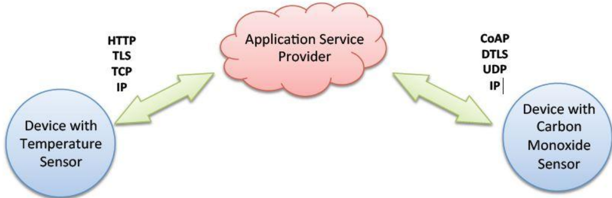
Fig 2: Device-to-cloud communication model diagram.
