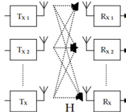
Figure 1: Schematics Representation Of A MIMO Communication System
