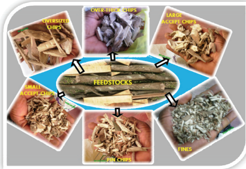
Figure 7. Chip samples classified
