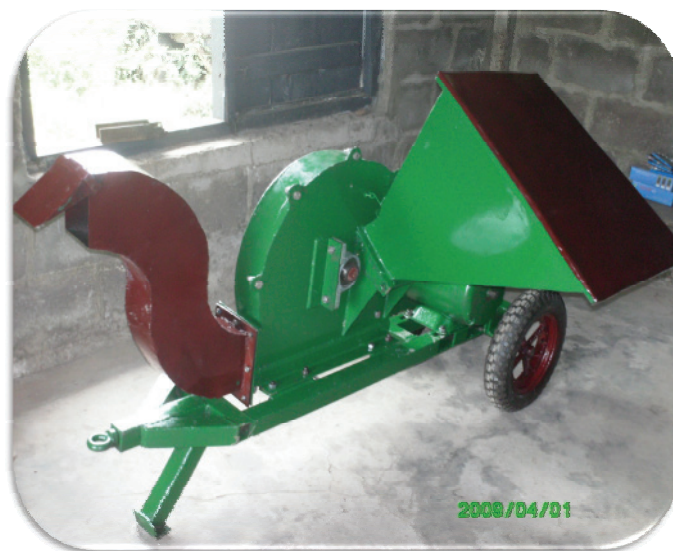
Figure 6. The mobile wood chipper
